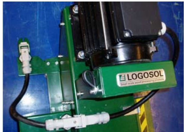
The log house moulder's cable with an additional plug as a safety breaker positioned over the cover.
